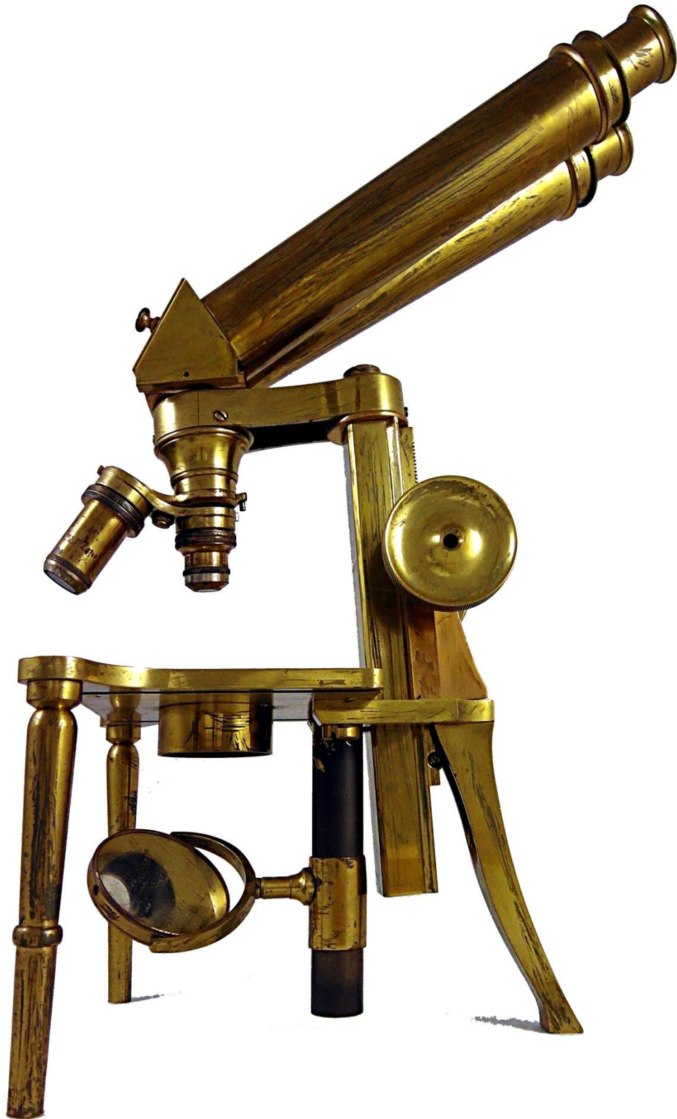
Figure 2. Riddell-Stephenson style stereomicroscope made by J. Swift and Son
