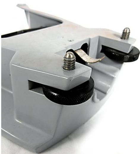
Figure 25. Thumb adjustments for locking screws on Transilluminating Substage Base, and illumination holder spring
