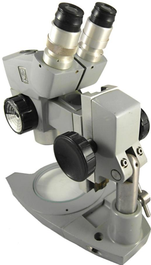
Figure 18. Series 59 in use, showing post receptacle with locking lever, and separated stage, segments. AO designated these two segments 59-851 and 59-852 respectively (shown here without stage clips).
