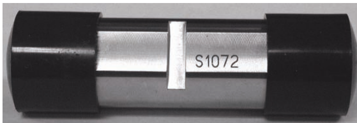
Figure 18. LightPipe flowcell with protective end caps, ready for storage
