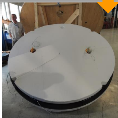
Epoxy resin impregnation under vacuum in a mold
