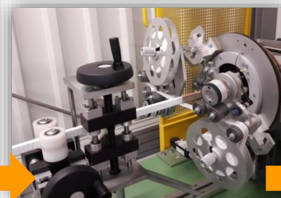
Sandblasting of the conductor followed by the wrapping of the fiberglass conductor insulation in a clean area
