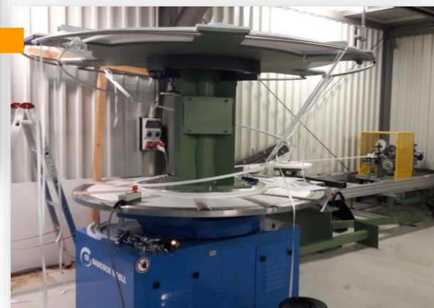
Winding the 1 st layer after having stored on the upper part the conductor length for the 2 nd layer
