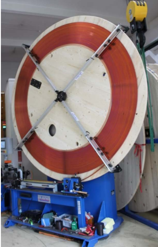
Fig. 4. Movable winding unit (in vertical direction) of total maximum height of 4.5 m. Each produced 265 m long RCOCC unit length is wound in a single pancake of 2 m internal diameter prior to their delivery to the coil winding manufacturer.
