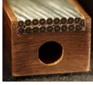
Fig. 1. Picture of the cross-section of the produced Rutherford cable on conduit conductor (RCOCC). The dimensions are 17.92 \times 12.96 \text{ mm}^2 .
