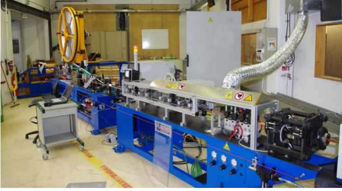
Fig. 3. First parts of the RCOCC production line including unspooling and straightening units, assembly and induction heating heads, crimping and calibration modules.
