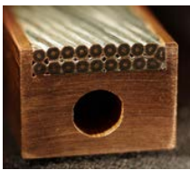
Fig. 2. Picture of the cross-section of the Rutherford cable on conduit conductor (RCOCC) produced. The dimensions are given in Table I.
