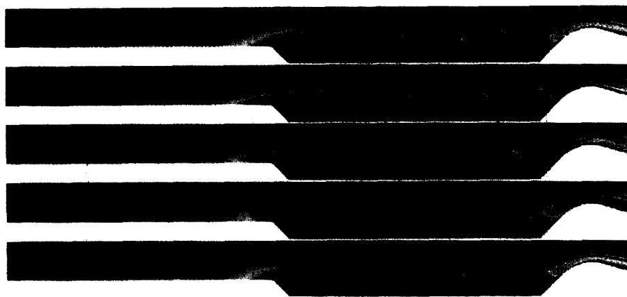
Fig. 14. – Contour maps of entropy at 5 equally spaced instants, in a low-Reynolds number 2D pseudo-DNS.
