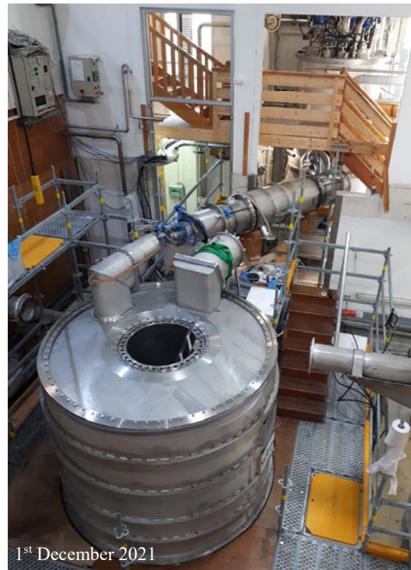
FIG. 1. LNCMI site dedicated to the hybrid magnet with the magnet cryostat assembly containing the large bore superconducting coil outsert, the cryogenic line ready for busbar insertion prior to its interconnection, and in the back, the cryogenic satellite producing the superfluid He.
