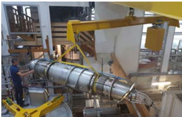
FIG. 1. Delicate handling operation of the cryogenic line in the hall of LNCMI-Grenoble with dedicated lifting tool.
