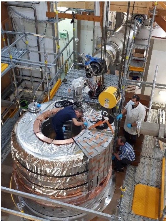
FIG. 1. Cryostatting step with the assembly of the 40 K thermal shield. The cryogenic line connecting the magnet cryostat to the cryogenic satellite is visible in the background.
