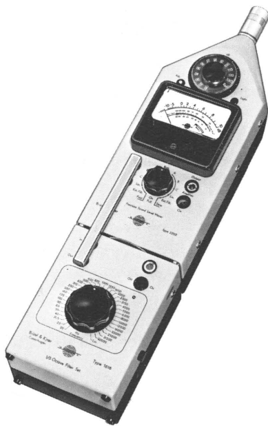
Fig.3.2. The 1616 mounted on the Precision Sound Level Meter Type 2203
