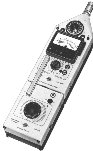
Fig.3.3. The 1616 mounted on the Impulse Precision Sound Level Meter Type 2209
