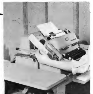
Edge-Punched Cards are filed for ease of selection for insertion into the Flexowriter for document preparation.
