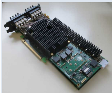
Figure 5: The PCIe40 card
