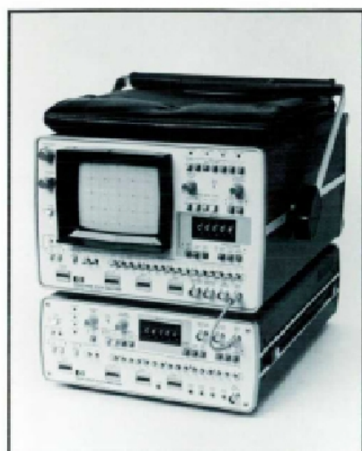
Fig. 3. Models 1600A and 1607A Logic State Analyzers work together to monitor and display 32-bit words, or work with independent clocks to examine the interaction between two digital machines. The combination of the two instruments is known as the Model 1600S. Model 1607A has most of the capabilities of Model 1600A and can work by itself using an oscilloscope or CRT monitor for the display.
