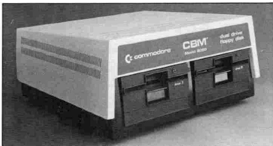
Figure 1-19. CBM 8050 Dual-Drive Floppy Disk Unit
